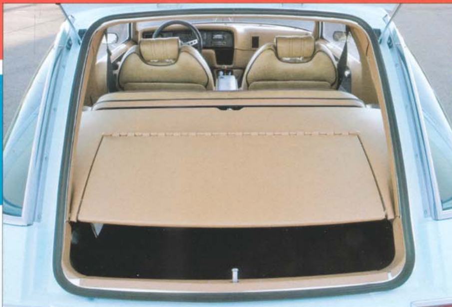
It's not called a fishbowl for nothing: All those windows allow anybody to see your stuff, so a cargo cover made sense. But all those windows also let in plastic-destroying UV rays, which makes the cargo covers an incredibly rare find today.
