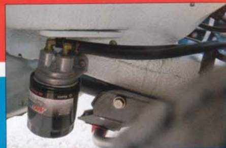
Perhaps dual remote oil filters on the 258 are overkill, but the Pacer didn't make it to 300,000 miles on luck alone.
