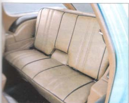
Hard-won original cloth seat covers deteriorated rapidly under sun exposure, so Buddy chose vinyl when reupholstering.
