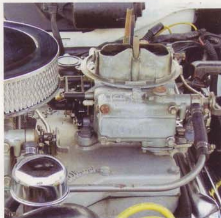
Every S/S AMX featured a specially built 390 with Crane-modified heads and a dual-carburetor Edelbrock intake manifold with 650 CFM Holleys
