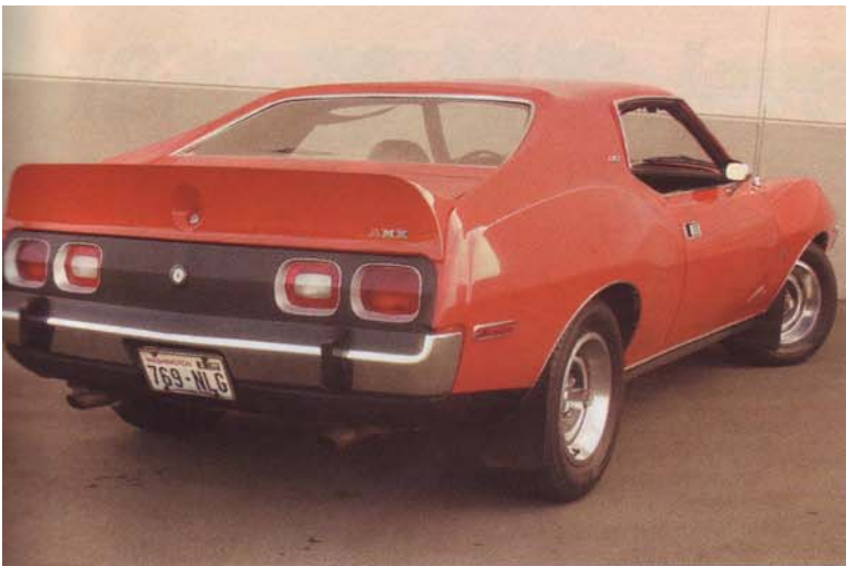
Metal under rear window and under wheel arch trim is rust-prone
