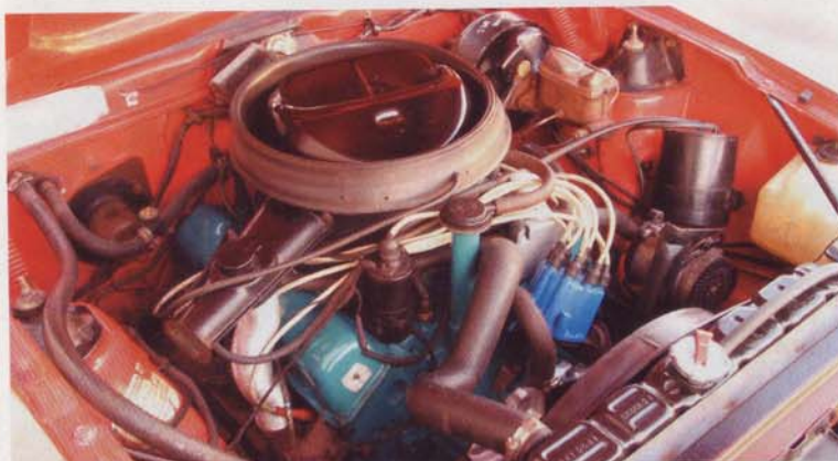
1970s AMC V-8s differ in bore size, but blocks are virtually the same
