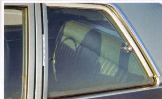
Glass is not unique to SC/360; it can be swapped with any Hornet two-door sedan's glass.
