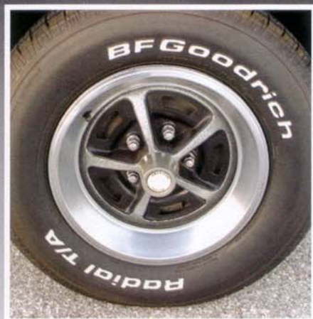
Fourteen-inch styled steel wheels were available as an option over the eight-slot wheels.
