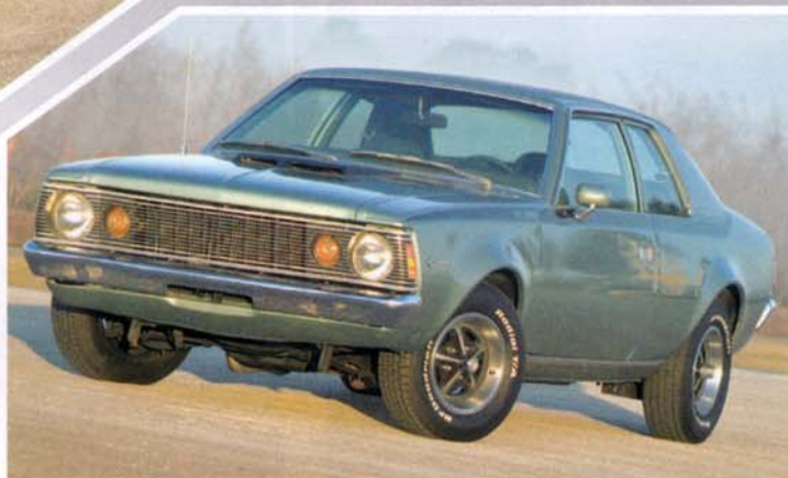
The SC/360's big exterior differences from a bog-standard Hornet two-door sedan include the subtle stripe and unsubtle hood scoop.
