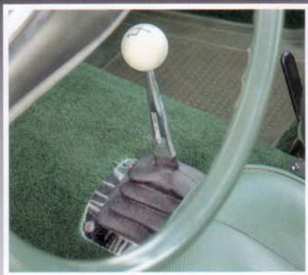
Hurst shifter stirs T-10 four-speed; also available were a three-speed manual and M-12 automatic.
