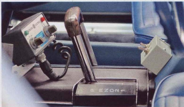
Add-ons for patrol duty were minimal: just the old-style growler siren, the single roof-mounted Dietz lamp, a control box and a GE Progress police radio
