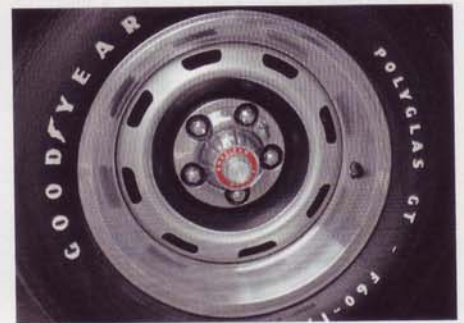
ADPS mechanics preferred the later eight-slot wheels and F-series tires because earlier wheels had a tendency to rust and E-series tires hydroplaned
