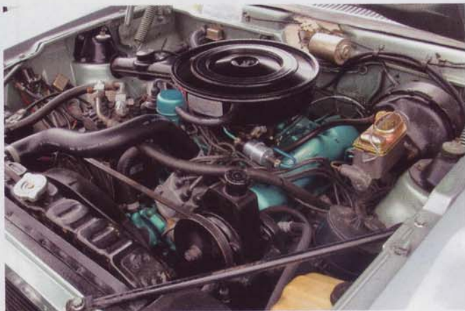
All police Javelins got the 330hp (255 net) fleet-duty 401-cu.in. V-8 from the Ambassador, along with air conditioning for those hot Alabama afternoons
