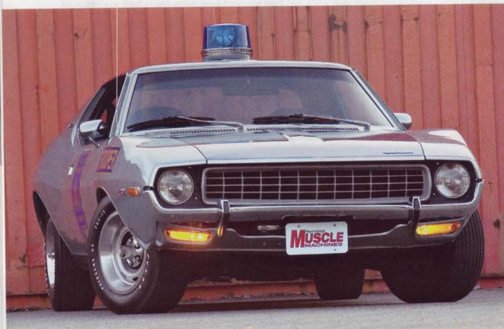
ADPS mechanics preferred the later eight-slot wheels and F-series tires because earlier wheels had a tendency to rust and E-series tires hydroplaned
