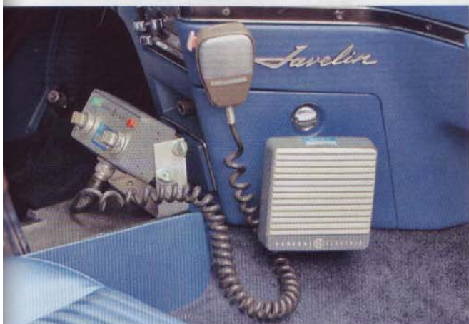
Add-ons for patrol duty were minimal: just the old-style growler siren, the single roof-mounted Dietz lamp, a control box and a GE Progress police radio
