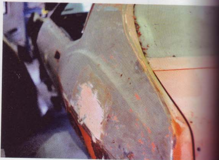
Stripping the paint revealed no major dents or damage; minor dents and rust repair areas were given a thin coat of Evercoat filler
