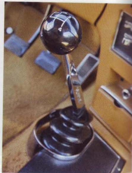
Hurst shifter stirs Borg-Warner T-10 four-speed, which remained untouched during the resto
