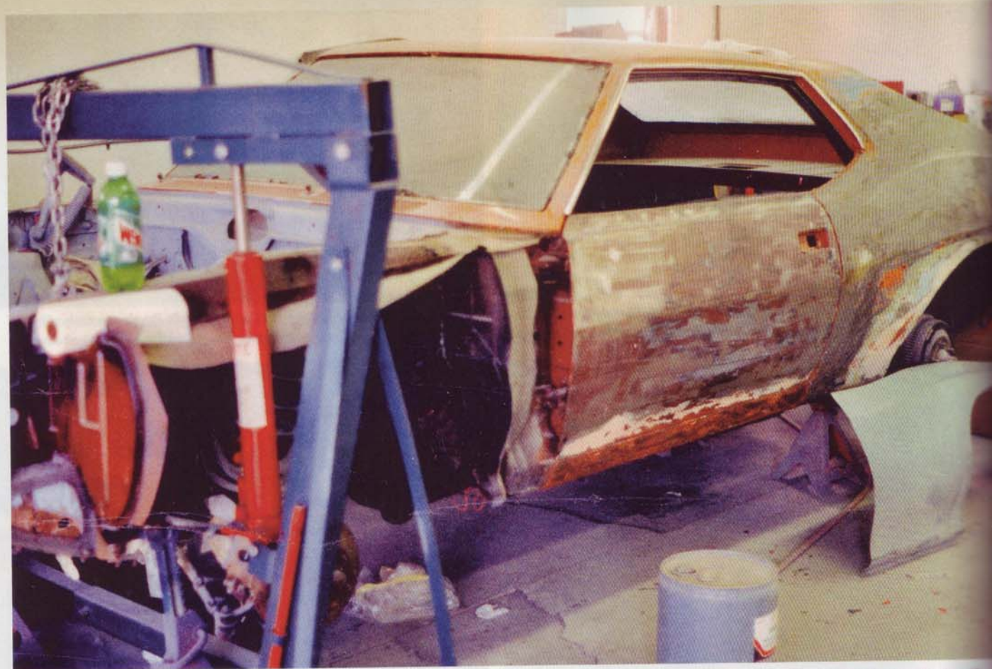
Shortly after the XMA arrived at the restoration shop, the body was stripped of its poor 1981 repaint using Klean-Strip paint stripper.
