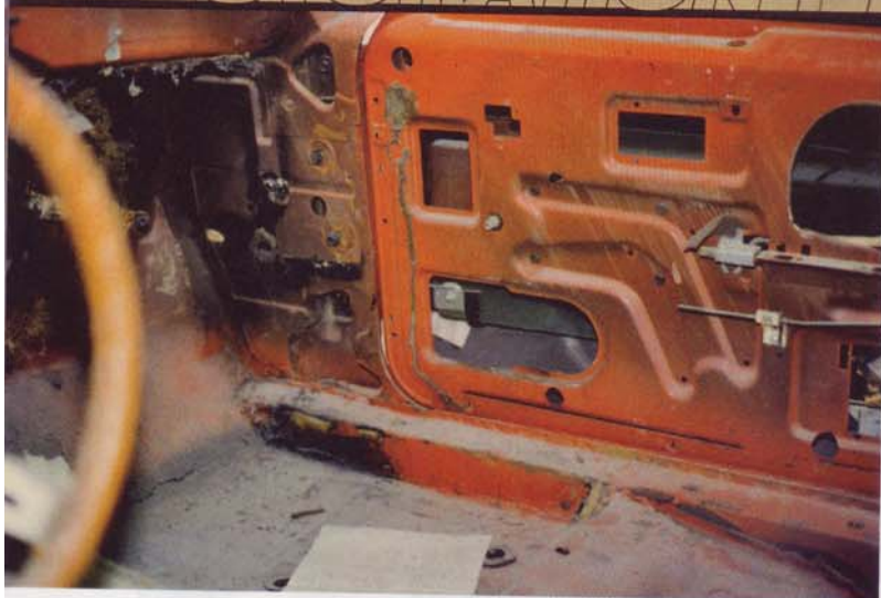
With the door panels off, the current owner could see where the rustproofing that the original owner had applied went inside the doors
