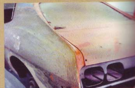
Only the quarter-panel sections behind the rear wheelwells rusted enough to warrant patches
