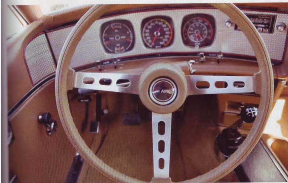
Engine-turned dash overlay took several years to find so owner could replace original overlay
