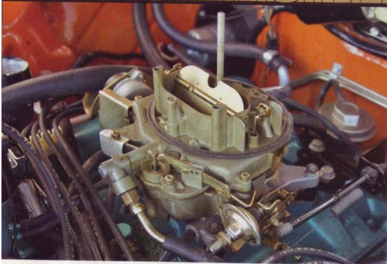
Though the owner replaced the Motorcraft 4300 four-barrel carburetor with an Edelbrock in 1991, he wisely held on to it over the years
