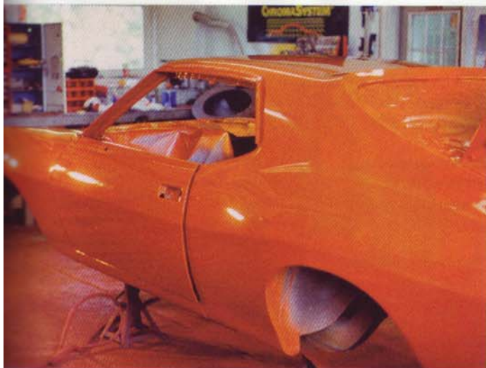
Another four coats of single-stage Valspar Sunthane polyurethane paint went on smooth after all the block sanding of the primer
