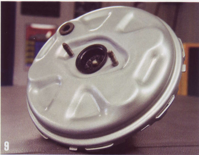
9 The finished product, just before re-installation. We've read tips about applying a final light "dusting" of blue metallic paint to further the impression of a cadmium finish, but decided the booster looked pretty good as-is, and elected to install it.
