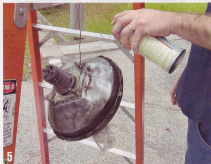
5 Eastwood's PRE is an aerosol paint prep material that cuts through grease and grime. We sprayed the booster and wiped it down. In any deep crevices, we used compressed air to blow out any residual material.
