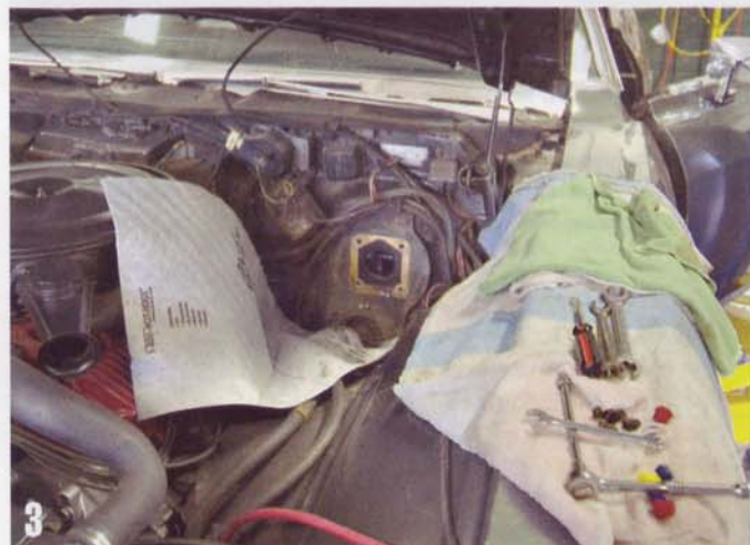
3 The biggest challenge in this whole project was getting the booster off. Full-size Buick boosters mount directly through the firewall with four nuts under the dash. They're tricky to get to, but we used a universal joint, a deep \frac{5}{8} socket and a 4-inch extension to get at them. The trouble was getting the booster disconnected from the pedal. After removing the cotter pin, we couldn't seem to get it to come off the clevis pin on the brake pedal. With a lot of wiggling, and liberal application of PB Blaster and profanity, it finally dropped off.
