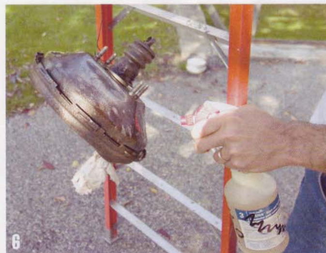
6 As a final step before primer, we mixed up a quart of Eastwood's Metal Wash, which comes in a fine powder. Five tablespoons of material plus a quart of warm water makes up a sprayable solution that promotes primer adhesion to bare metal.
