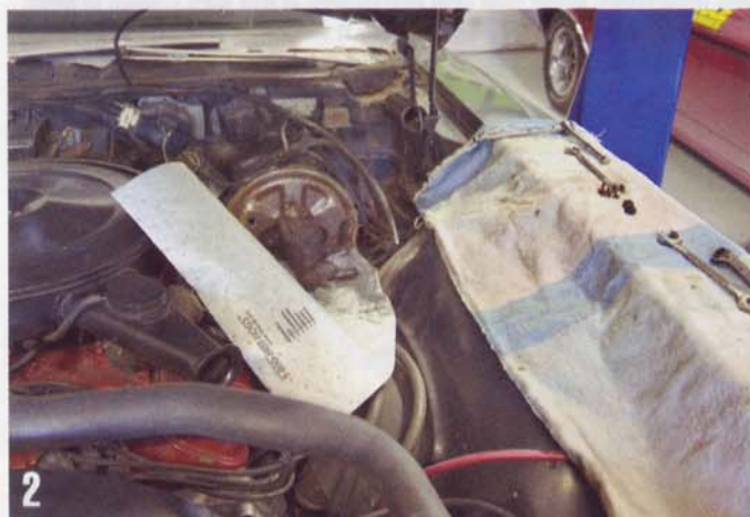
2 The master cylinder separates from the power brake booster with two nuts. We also removed the windshield washer reservoir for better access to the booster.
