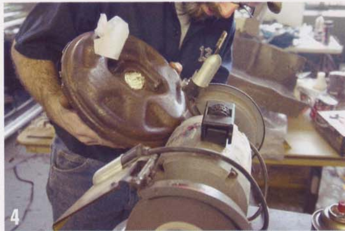
4 We have access to a media blasting cabinet, but the idea of abrasive material flying around inside the booster's diaphragm wasn't too appealing. We plugged whatever holes we could find and went at the surface rust with a wire wheel and wire brushes.
