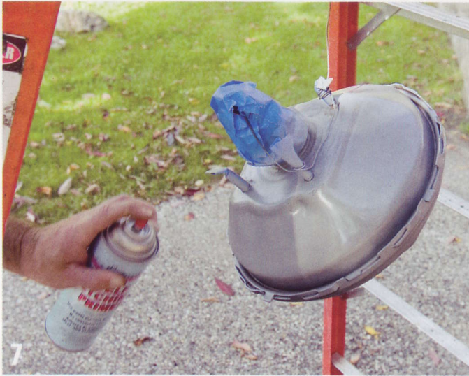
7 After thoroughly drying the booster, we applied two coats of Eastwood's Self-Etching primer and then allowed it to dry for a couple seconds—it dries almost as fast as it comes out of the can, perfect for a time-crunched hobbyist.
