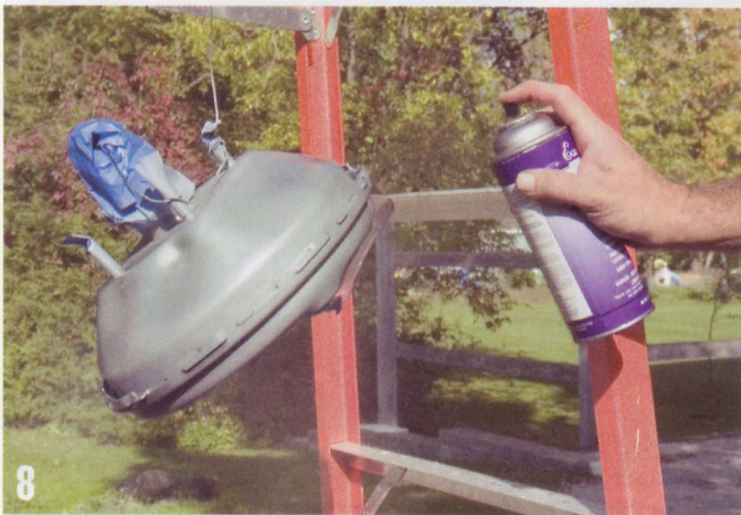
8 The Silver Cad paint is a mix of silver paint with silver, green and blue metallic highlights that gives the appearance of silver cadmium plating.
