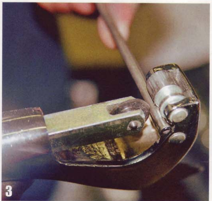
3 Practice making smooth cuts using a proper tubing cutter. Make sure to dress the finished surface and remove all burrs.
