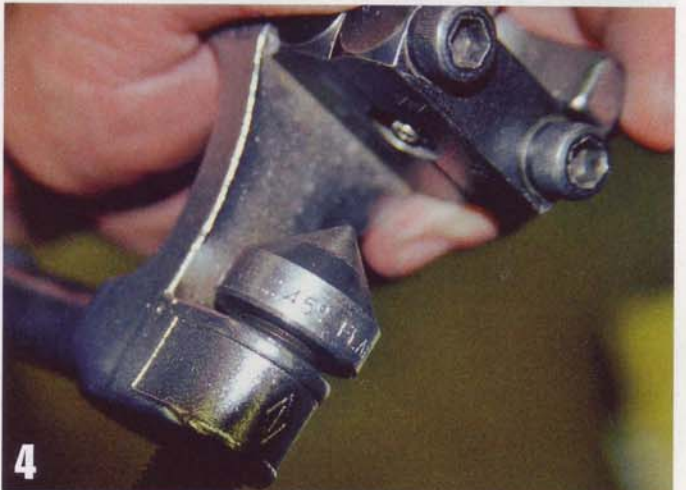
4 The tool will identify the type of flare. This example is a 45-degree flare.
