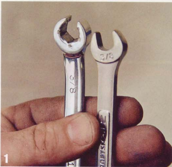
1 A line wrench (left), also known as a flare-nut wrench, is used to break loose or tighten the fitting. Once the fitting is loosened, a conventional open-end wrench can be employed.
