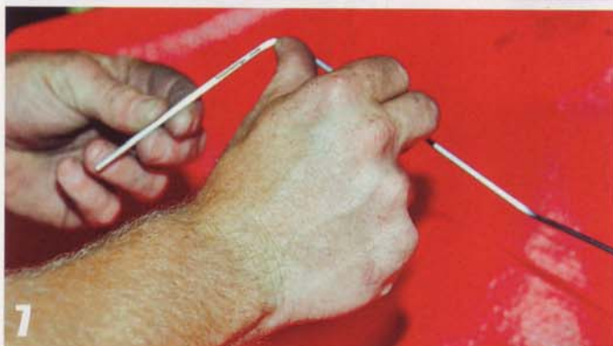
7 In most instances, the best template is the old line itself, such as the Mopar fuel line (above). To fabricate a template, welding wire is a good choice because it's easy to work with.
