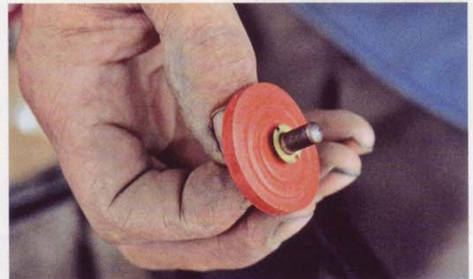
Once the coil is removed, the carbon button can be accessed. When installing a new cap, do not forget to install the new carbon button. Many leave the button out and the coil arcs to the rotor through the hole. The engine will start this way, but will misfire in a few miles.
