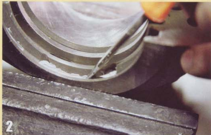
2 He then distributes the silicone evenly around the receiver groove for the rear main seal.
