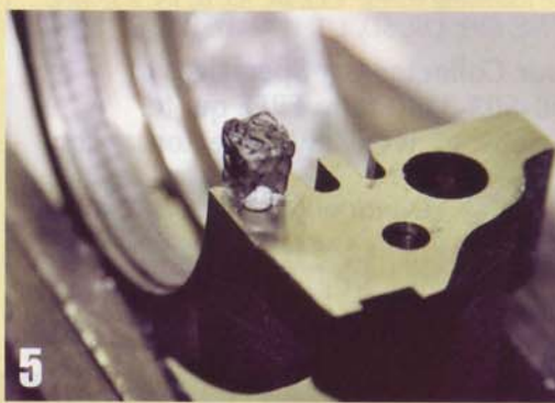
The wick seals are longer than required and need to be trimmed. Note the small amount of silicone protruding from only one side of the seal.
