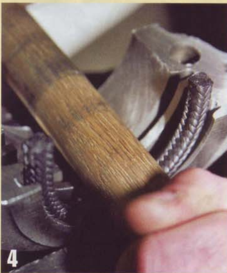
The Best Gasket GraphTite wick seal is then pressed into place.
