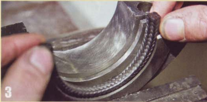
The Best Gasket GraphTite wick seal is then pressed into place.
