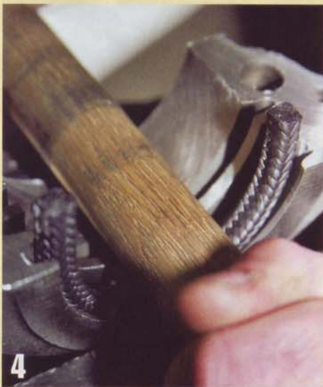
3 The Best Gasket GraphTite wick seal is then pressed into place.
