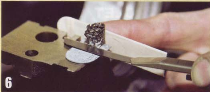
Best Gasket recommends that the GraphTite material should protrude 0.015 inch above the surface. The company provides a spacer, razor knife and finger shield to easily accomplish this.
