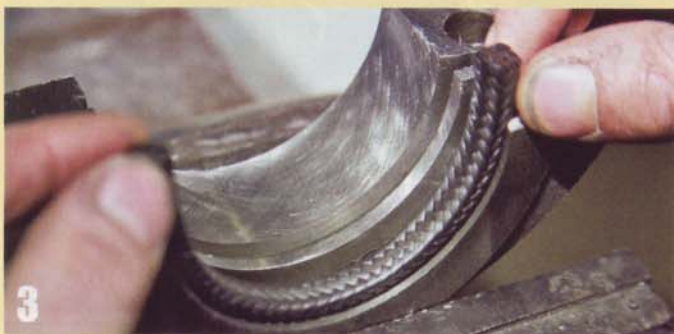
3 The Best Gasket GraphTite wick seal is then pressed into place.
