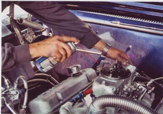
Carburetor cleanliness is very important for proper operation. This carburetor was very black in the venturis, usually a sign of backfiring/popping through the intake when cold.
