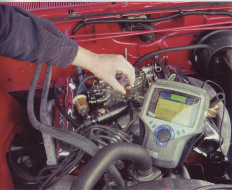
The OTC/SPX Performance Gas infrared exhaust gas analyzer being used to "read" the air/fuel mixture as the idle mixture is being set on this '68 Fury III's 383-cu.in. V-8.
