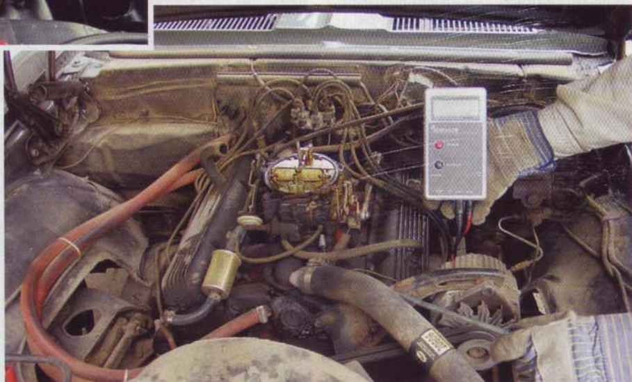
Air-fuel mixture being checked and set on a '68 Camaro's 327 using the Innovate Digital meter
