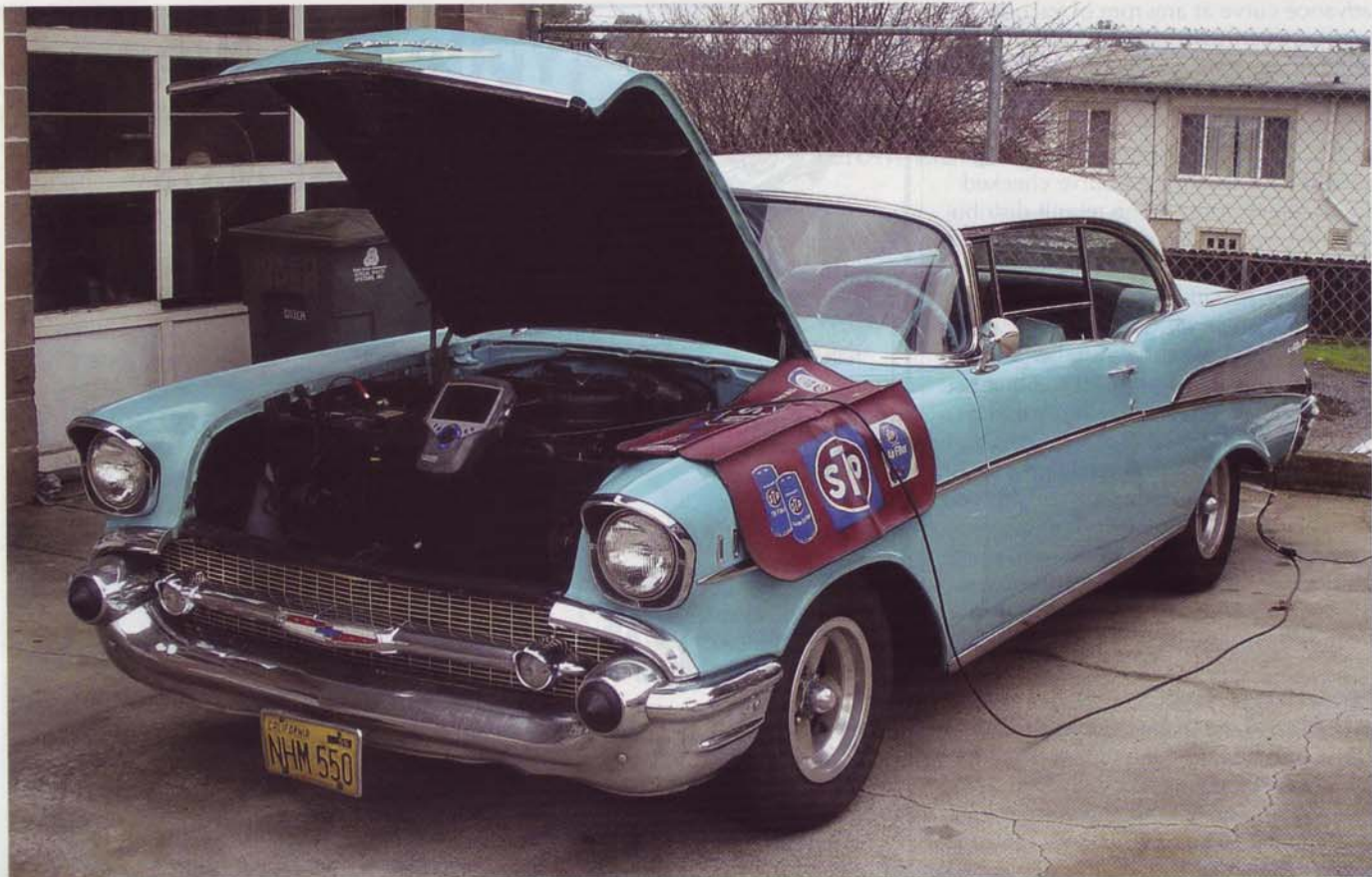
With the engine running, the safest way to test this 1957 Chevy's air-fuel mixture using an infrared exhaust gas analyzer is outdoors
