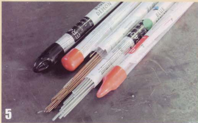
5 A variety of rod thicknesses is a must, but we’ve so far stuck with ER4043 (the silver stuff) on aluminum and ER70S6 (the copper coated stuff on steel). The ER stands for electrode/rod, the next two numbers denote the filler’s tensile strength (40 equals 40,000 p.s.i.; 70 equals 70,000 p.s.i.)
