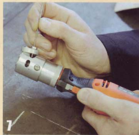
You can sharpen tungsten electrodes on a bench grinder with a dedicated wheel, but once you use HTP’s Tungsten Grinder (about $239.95), you’ll never go back. It not only sharpens the tungsten quickly and accurately, but it can cut and flatten tungsten as well. Great tool.
