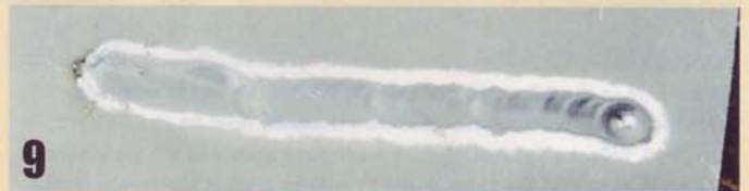
9 This is a bead our man ran on light-gauge aluminum with no filler rod. It started out way too hot but ended up okay. We’d give it a C-plus.
