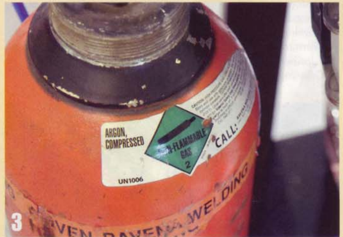
3 Argon is used as a shielding gas in TIG welding for almost any application. Helium was originally used in TIG welding, hence the Heliarc name, but was edged out for a few reasons. Among them, helium is more expensive than argon and must be used in greater volume.
