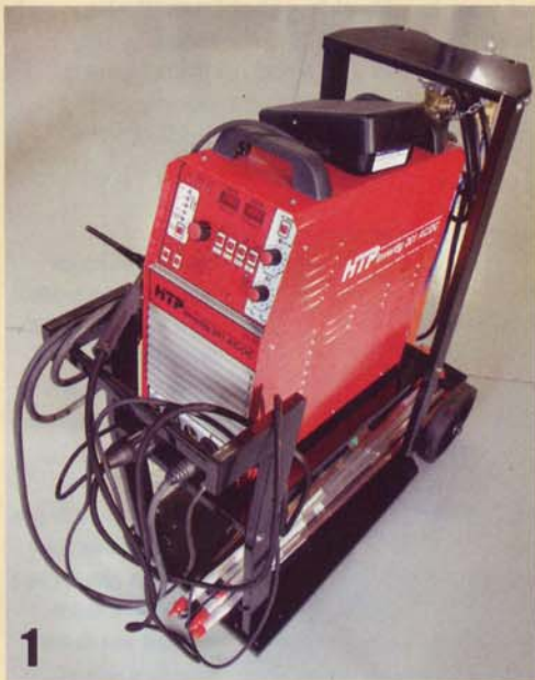
1 The official TIG welder of Hemmings' shop is the HTP Invertig 201 AC/DC from HTP America Inc. It sells for $2,395 without the cart and is a full-featured inverter-based TIG with pulse and variable AC frequency. It weighs just 68 pounds, is about the size of a desktop computer and draws just 30 amps from the 220-volt outlet.
