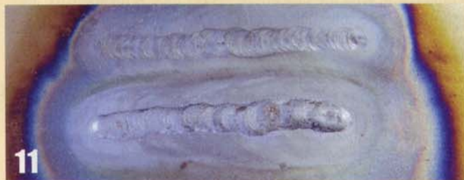
The top bead was run on 20-gauge sheetmetal with no filler. Not bad. The lower bead was run with ER70S6 filler rod with reasonably good results. The bead starts well but gets a little shaky and hot as the welder progressed to the right. Practice, practice, practice. B-minus, and that's being kind.
