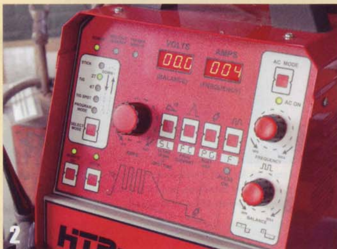
2 Shown here in the AC mode, our Invertig 201 allows you to adjust the AC balance from 10 to 90 percent and the frequency from 20 to 200 hertz. In a nutshell, balance determines how much heat goes into the work versus how much goes into the torch, while frequency control allows you to dial in the width of the arc cone from a wide arc at 20 hertz to a pinpoint-narrow 200 hertz.
