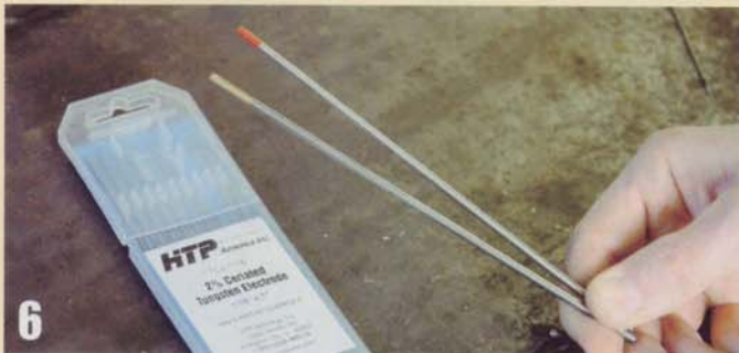
6 We’ve been using 2 percent ceriated tungsten (the package in the background) from HTP, which can be identified by a gray tip. It works well in AC and DC modes on a variety of materials and isn’t radioactive. The red-tipped tungsten is 2 percent thoriated. It’s widely used, most commonly in DC mode, and works well on steel and stainless steel but does carry a low-level radiation hazard. The gold-tipped tungsten is 1.5 percent lanthanated, which can be used in AC or DC modes with any type of machine, whether inverter- or transformer-based.
