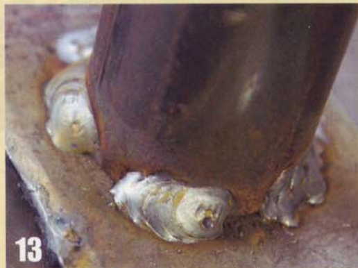
And here's a similar setup TIG-welded with the Invertig 201. There's nothing wrong with the MIG welds, but the TIG weld is definitely more uniform and aesthetically pleasing. 🔧
