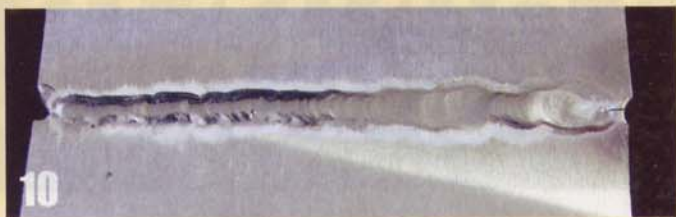
This time we added some ER4043 filler rod, and the results were so-so. The weld starts out pretty good (notice the shine), but at about the halfway point, the material became overheated and our man never compensated by backing out of the pedal. The rest of the bead (from the center to the right) is too hot.
