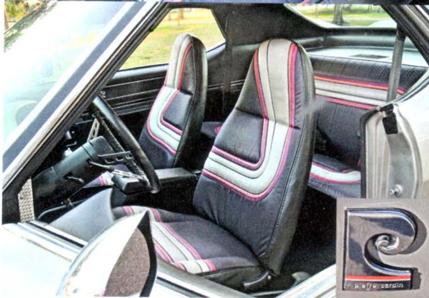
The wild Pierre Cardin interior wakes up the AMX's interior. The wraparound instrument panel is faced in engine-turned aluminum and is equipped with the optional Rally Pac. The three-spoke sport wheel and tilt steering column were also extra cost. When the optional Pierre Cardin interior was ordered, these emblems (inset) appeared on the front fenders and the interior door panels.
