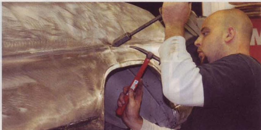
18 That stud was used as an attachment point for the Morgan Nokker. The slugger was inserted over the stud, and the metal was worked out to eliminate low area.
