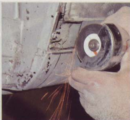
4 The 3-inch cutoff wheel went to work to remove the rusted metal.
