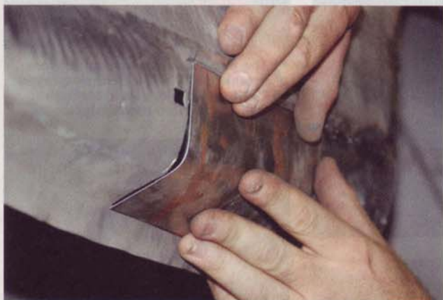
11 Rather than having one big patch, smaller patches were used in order to more accurately follow the factory shape along the bottom of the quarter-panel.
