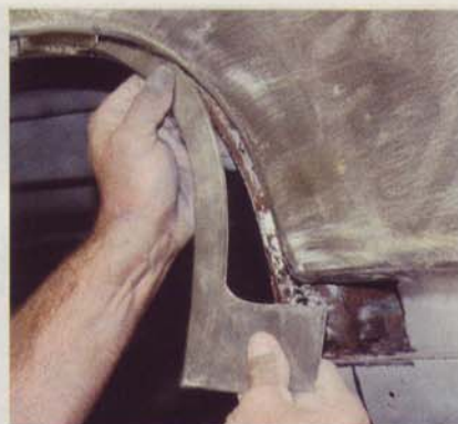
6 Jelinek checked the patch's fit before doing final trimming and deburring.
