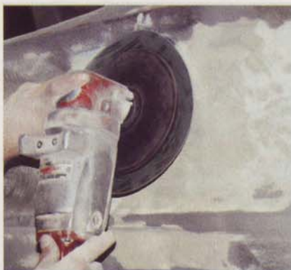
1 At first glance, the Nova's passenger-quarter's overabundance of filler suggests major dents and damage. Bill Jelinek of Rt. 66 Motorsports thought otherwise and set out to uncover the actual condition of the metal by buzzing the filler off the panel with an 8-inch grinder fitted with 3M 24-grit 9-inch discs.
