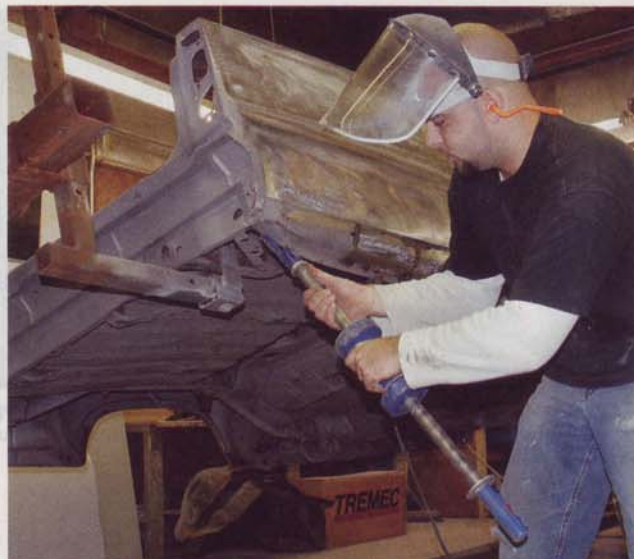
13 Rock worked the metal in the corner using the dent-removing slide hammer, technically called a Morgan Nokker, but more commonly referred to as a slugger. The weight slides down the shaft and strikes the handle, creating a pull on the panel. This process is time-consuming but very effective for removing dents.
