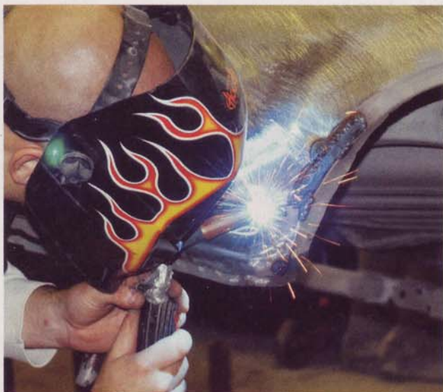
10 Moving back to the rear quarter-panel, Kevin Rock took over and continued the careful process of metal repair.
