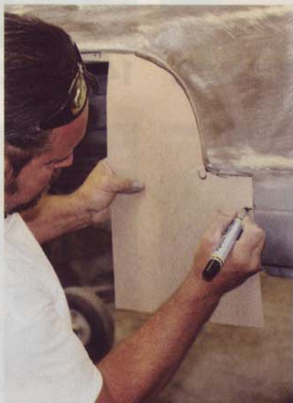
5 Using a piece of cardboard, Jelinek created a template for the sheetmetal to be replaced. Next, he traced the shape he needed and cut the patch from 18-gauge metal.
