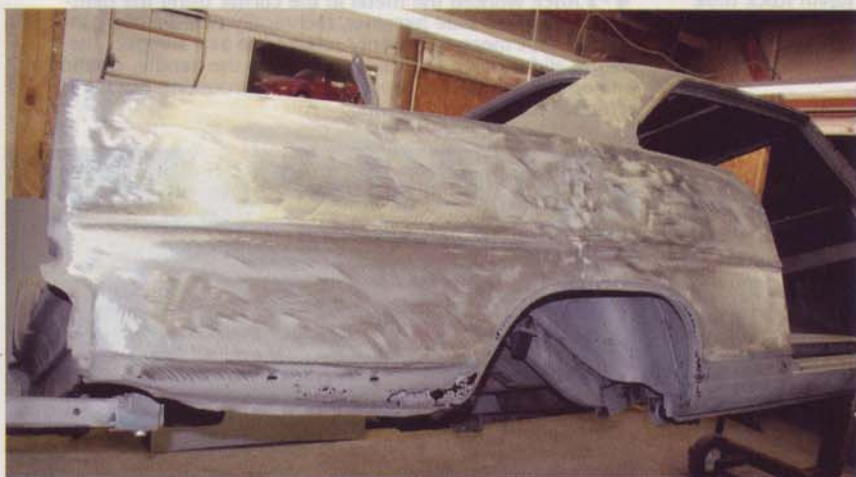
2 After the filler was removed, three trouble spots became evident: a fairly large, low area directly above the tire; a low spot near the Super Sport emblem location and a dent in the rearmost bottom corner of the quarter. The rust along the bottom of the quarter and wheelwell lip is minimal and can be easily repaired.
