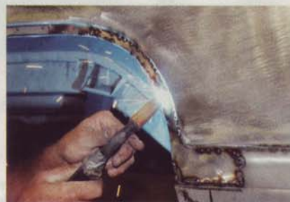
8 The rocker/wheelwell lip patch was MIG-welded to the car. It was first tack-welded to ensure proper fit, then finish-welded, with Jelinek taking care not to overheat the surrounding metal.
